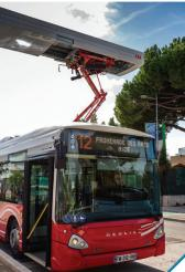
SNEF (PACA)/City of Nice: Pantograph to power the network of electric buses.
